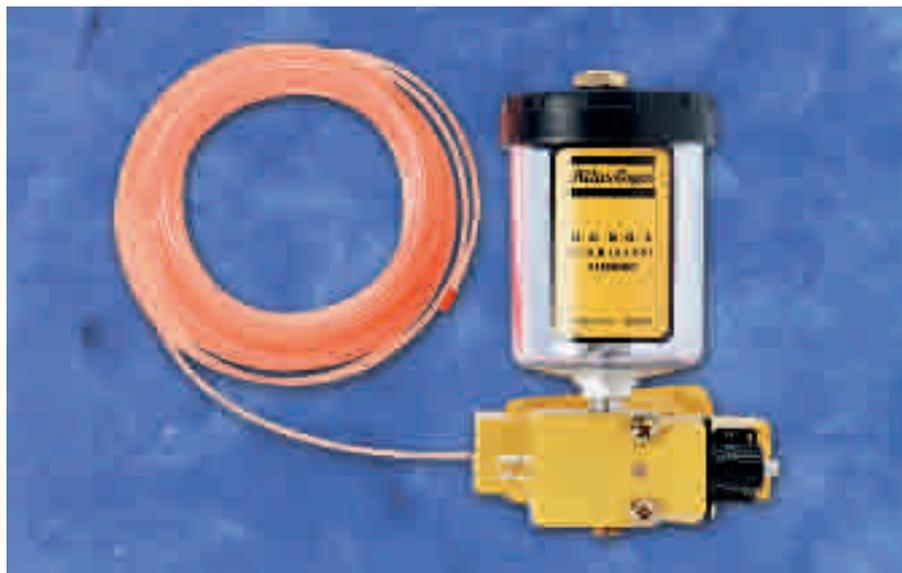
of oil in 40 steps (30 to 3 mm<sup>3</sup>). This helps to minimize the oil dose. Every DOSOL SPL unit includes as standard a counter with a switch that allows the lubricator to operate every first, fifth or tenth tool cycles.
