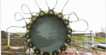
CTST tensioning tools are supplied with two hydraulic connections. This allows for very simple link hose configuration to link multiple bolt tensioning tools together.
