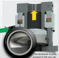
culated Bolt load is directly proportional to hydraulic pressure. The bolt stretches and a gap is formed below the hexagon nut. Once the target pressure is reached, the pressure is
