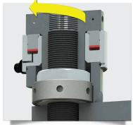
The thread insert (puller) is screwed onto the bolt
