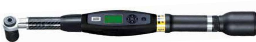
BI controller is the new controller with the battery inserted in the STwrench handle. New batteries are to be used only in this controller. Recharge these batteries using standard battery charger with BI battery charger adapter.
