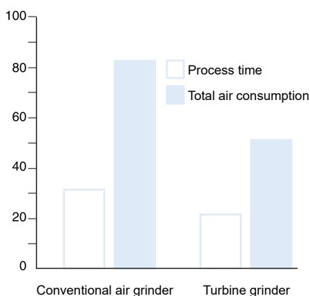
*The turbine motor is more efficient than a conventional grinder motor. Therefore it takes less time to do the same job. Also the total air consumption will be a lot less for a specific job.*
