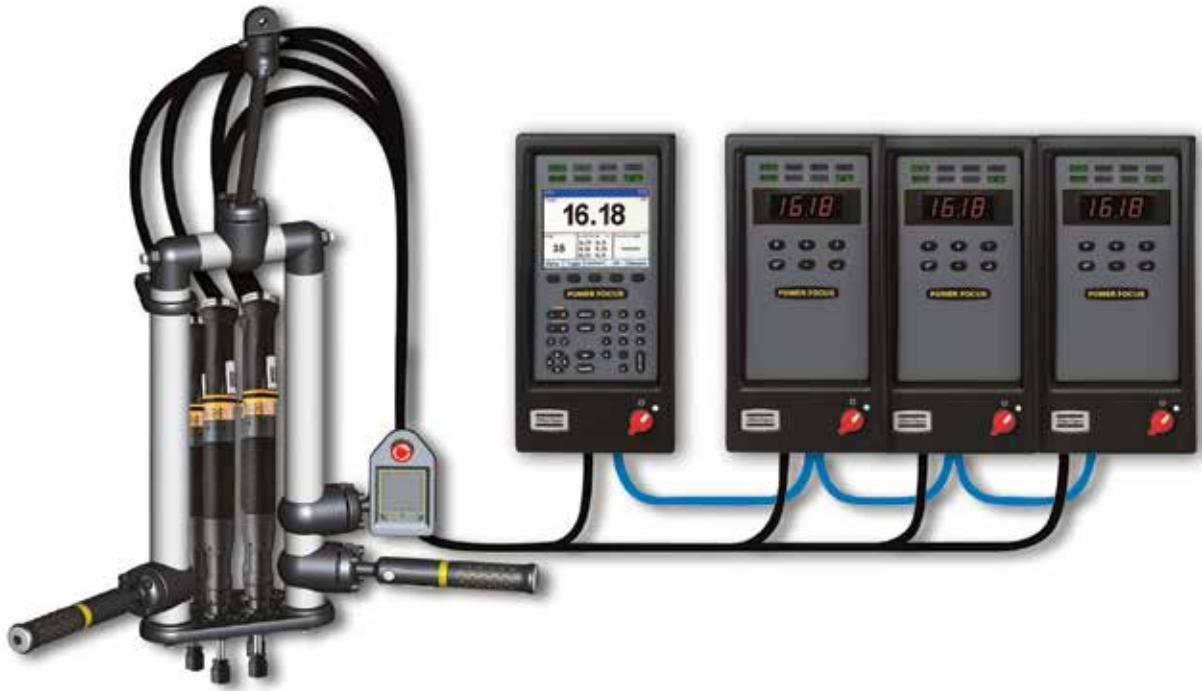
Tensor spindles are easily fixtured using our standard range of Express mechanics. The control strategies StepSync and SynchroTork synchronize Tensor spindles to provide consistent clamp forces over the entire component mating face.
