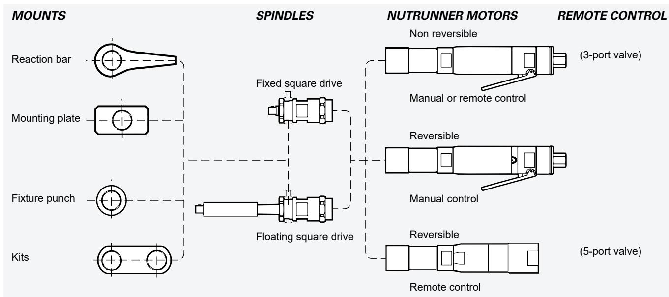
LTD28, 38 and 48 straight nutrunners are based on the power package and clutch from the LTV angle nutrunners.
