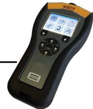
The device which connects the Load Cell with the Sta 6000
